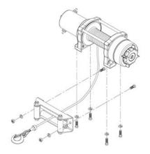
to make sure the motor, drum and gearbox housing are aligned correctly.
